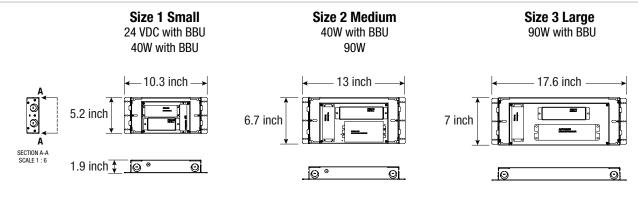
BBUX — Battery Backup & LED Driver Remote (Outdoor), IP67, IK10, NEMA 4X, -20 to 55 °C (-4 to 131 °F), 30 feet Maximum Distance with 12AWG (with UNV Option Only)
